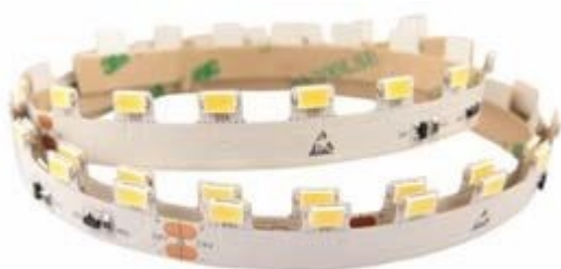
STRISCIA LED FLEX CIP LED 5630 ORIENTABILI NUMERO 70 METRO 24VDC 15 W METRO 1400 LUMEN METRO SEZIONABOLE OGNI 100 MM 2200K/2700K/3000K/3500K/4000K/5000K/6000K CIRCUITO H10MM A MARCHIO CE
